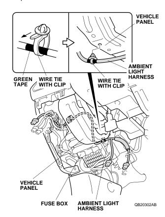
10. Using diagonal cutters, cut the clip portion off of one wire tie.
