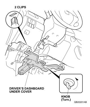
4. Remove the driver's dashboard lower cover (nine clips and unplug the vehicle connectors).
